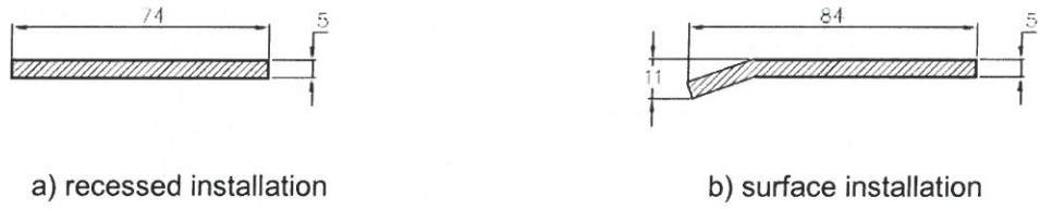
Fig. A3. CONECTO PARK SL waterproof expansion joints profiles – stainless steel
